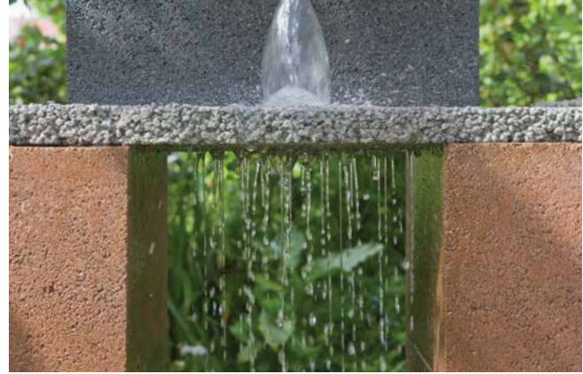
Instead of running off, water flows right through porous concrete. Source: JJ Harrison .
