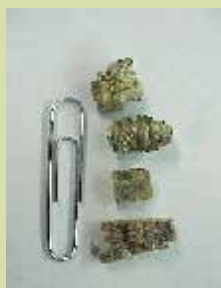
Vermiculite insulation is often nugget-shaped and silver-gold or gray-brown. Source: Agency for Toxic Substances & Disease Registry
