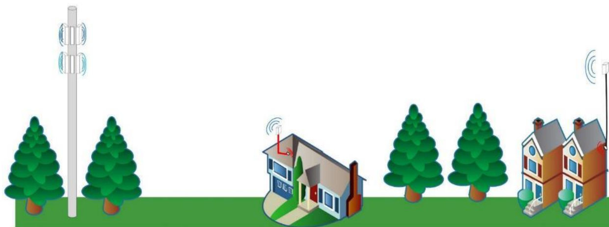
Figure 38: Example Fixed Wireless Network with Antennas on a Monopole and Customer Premises
