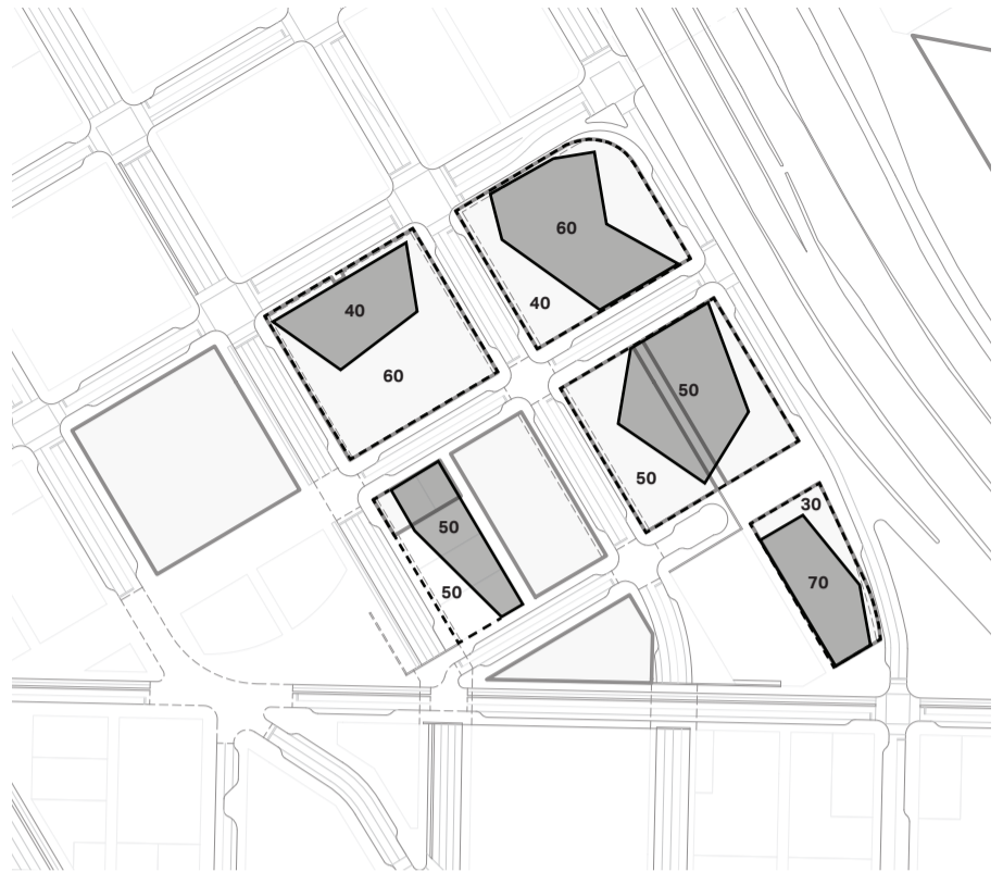
Maximum lot coverages and minimum open space areas in the Courthouse District.
