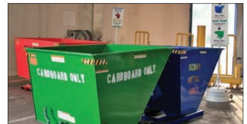
Bins are color-coded – green for cardboard, blue for scrap metal, and orange for clean wood – so customers can sort out recyclable materials.
